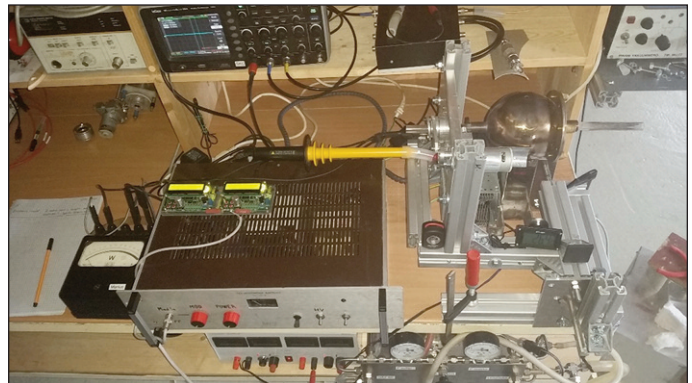
Photo 7. Spherical transverse magnetic cavity resonator made of steel plate.
