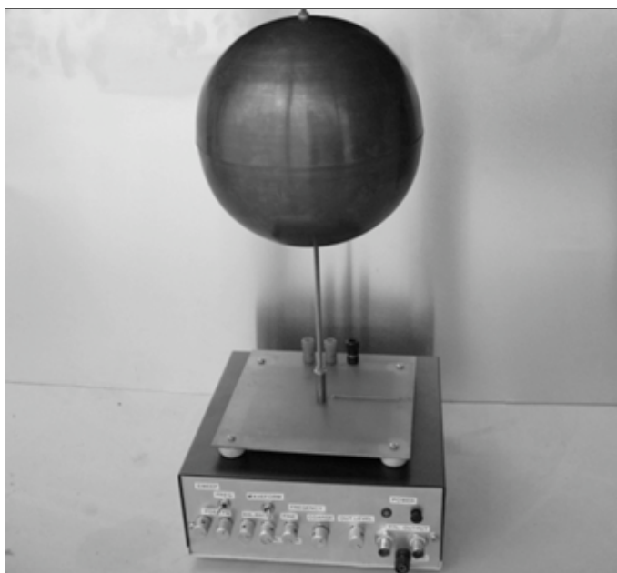
Photo 3. Tesla-wave generator for calibration 100 Hz -1 MHz.
